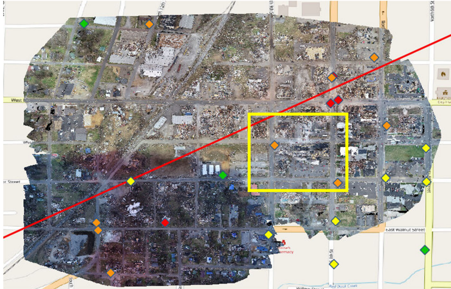
Figure 2. Screenshot of QGIS (within DesignSafe) showing drone imagery from Mayfield, Kentucky (Pilkington et al., 2021) along with NOAA Damage Assessment Toolkit (DAT) data points (NOAA 2021). The yellow box has been added to indicate the view that is enlarged in Fig. 3.
