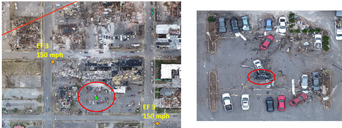
Figure 3. Left: Enlarged view of a portion of Fig. 2 showing drone imagery (Pilkington, et al., 2021) overlaid with NOAA DAT data points (NOAA 2021). The green dot denotes the location of vehicles that were moved by the tornado. Right: Enlarged view of the area circled in red in the photo on the left.
